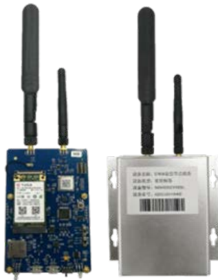
Fig.3 UWB anchor and tag two-in-one device
